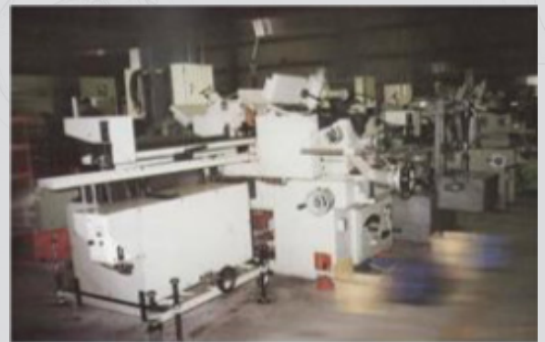
Centerless grinding machine with tandem linkage for 2-6 sets.
