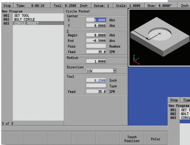
**FOUR** Tool paths are also displayed in 3D graphics that can be rotated and manipulated. The program is ready to run. Simply press “GO.”
